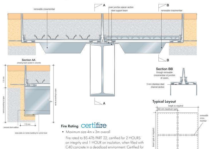
integrity only when finished with a tile, slab or stone infill
